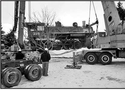
Cranes lift UP 535 from the display track in LaBonte Park in Laramie.
